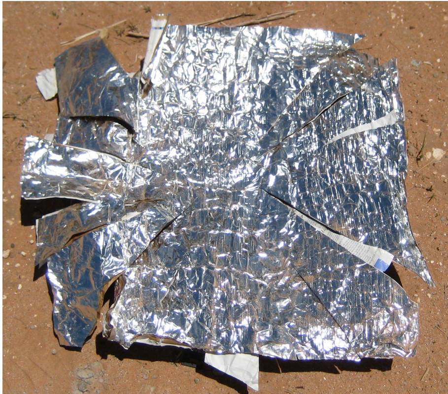
Cut wedge shapes so the plastic will conform to the shape of the dish.
